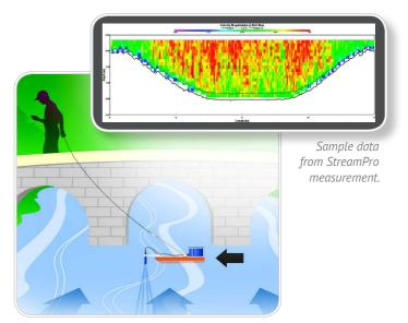
Teledyne RDI's StreamPro ADCP can simply be pulled across the stream as you walk across a bridge, or attached to a tagline to collect real-time data.
